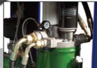
Dual Filtration & Oil Separator
